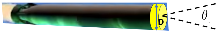
Figure 2: Sonar preliminary design task: Sonar (yellow) mounted on an Autonomous Underwater Vehicle (AUV), is circular array of diameter D with beamwidth \theta .
